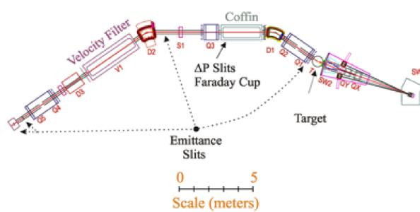
Figure 1. The MARS setup with the beam entrance and target on the right, and the detectors on the far left.
